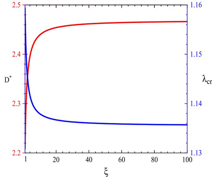
**Fig. 13.** The actual electric displacement  $D^*$  versus the dielectric constants ratio for the plate with  $c^{(f)} = 0.2$ ,  $\chi = 10$ , and  $\bar{D} = 2$  (red curve), and the critical stretch versus dielectric constants ratio for the DE laminate plate with  $c^{(f)} = 0.2$ ,  $\chi = 10$ , and when  $kH \rightarrow 0$ . The plate is subjected to the electric excitation  $D^* = 2$  (blue curve).
