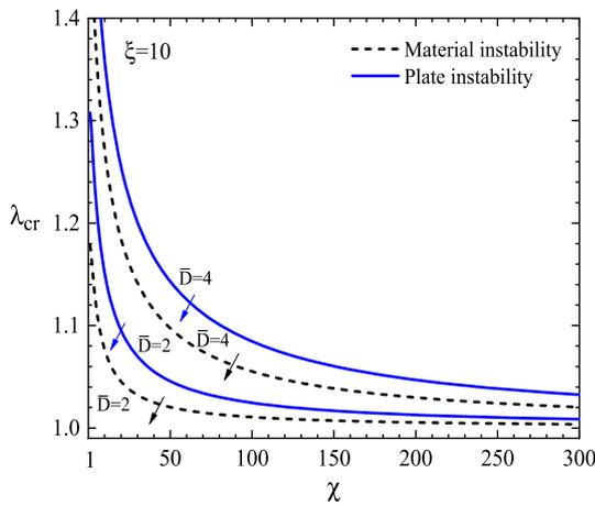
**Fig. 11.** The critical stretch versus the shear moduli ratio and  $\xi = 10$ , for the DE laminate plate with  $c^{(f)} = 0.5$ , and when  $kH \rightarrow 0$ . The plate is subjected to two different levels of the electric excitation:  $\bar{D} = 2$  and 4. The black and blue curves denote the macroscopic material, and plate instabilities, respectively. (For interpretation of the references to colour in this figure legend, the reader is referred to the Web version of this article.)
