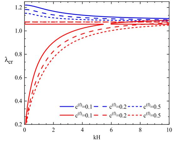
**Fig. 6.** The critical stretch versus the normalized wavenumber  $kH$  for the DE laminate plate with  $\chi = 10$ ,  $\xi = 10$  and different volume fractions  $c^{(f)} = 0.1, 0.2, 0.5$ . The plate is subjected to electric excitation  $\bar{D} = 2$ . The blue and red curves denote the antisymmetric and symmetric modes, respectively. (For interpretation of the references to colour in this figure legend, the reader is referred to the Web version of this article.)
