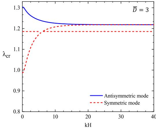
**Fig. 4.** The critical stretch versus the normalized wavenumber ( $kH$ ) for the DE laminate plate with  $c^{(f)} = 0.2$ ,  $\chi = 10$ ,  $\xi = 10$ . The plate is subjected to the electric excitation  $\bar{D} = 3$ . The blue and red curves denote the antisymmetric and symmetric bifurcation modes, respectively. (For interpretation of the references to colour in this figure legend, the reader is referred to the Web version of this article.)
